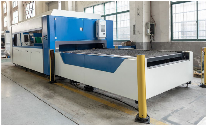
AWE 6kW CNC Fibre Laser (4m long x 320 ton)
